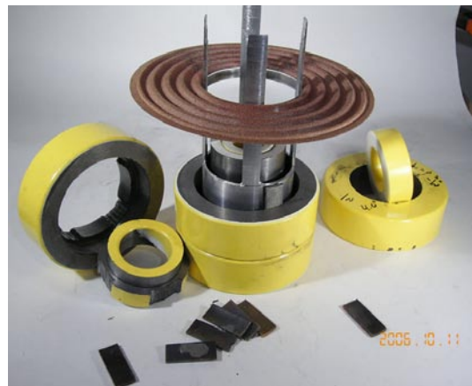
Figure 7 above shows 18 inch woofer motor structure.
