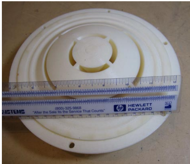
Figure 36 above shows the phase plug entrance slots.
