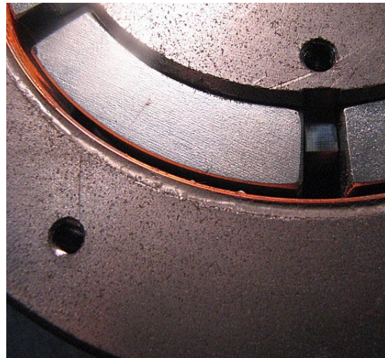
Figure 13 above shows a photo of the CID gap with primary and PM segments.
