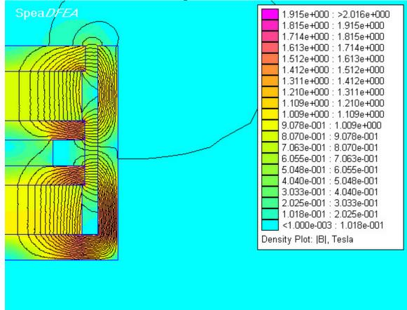
The Graph below shows the B curve including the LRRP gap. Both the upper and lower gap B's are .78 T. So the gaps will act symmetrically. The integrated B across the same 7.3mm coil is now .71 T for a 73% increase in B!
