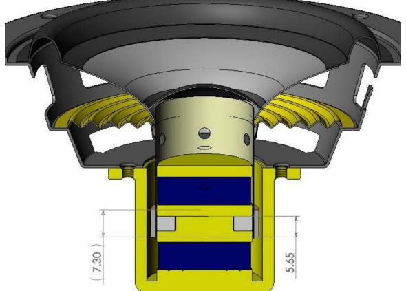
The physical Xmax for an MMAG motor is calculated by: (WH-Gapspace) / 2 + Gap. For this speaker the gapspace is 4mm and we know the coil is 7.3mm so
