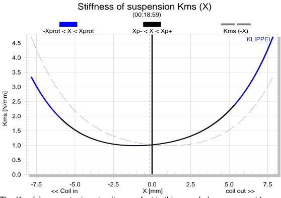
The Kms(x) symmetry is not quite a perfect in this sample however a spider geometry change will improve this in production units. Still, the total asymmetry on this sample is only 1.5mm.
