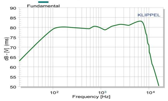
Fundamental + Harmonic distortion components Signal at IN1
