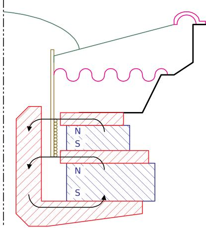
This provides two distinct advantages over conventional motor topologies. The first is that a much wider range of optimum coil height to plate thickness ratios can be achieved. (Think higher sensitivity *and higher Xmax*). The second is that the permeance coefficient of the motor can be optimized for a particular magnet material. (This means the most economical use of the magnet). For neo magnets this means a far more economical use of increases in magnet thickness.
