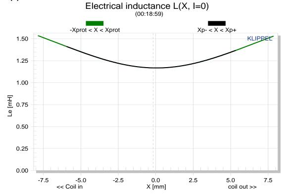
The non-linear inductance created by this motor system is virtually unique in speaker designs. Putting a shorting ring in the center of the virtual gap creates almost perfect symmetry, very low inductance and very low eddy currents in the steel parts. Klippel has shown that non-linear inductance is the most objectionable of the three non-linear components. The LRRP/MMAG motor reduces this component below the audible range even at maximum excursion.
